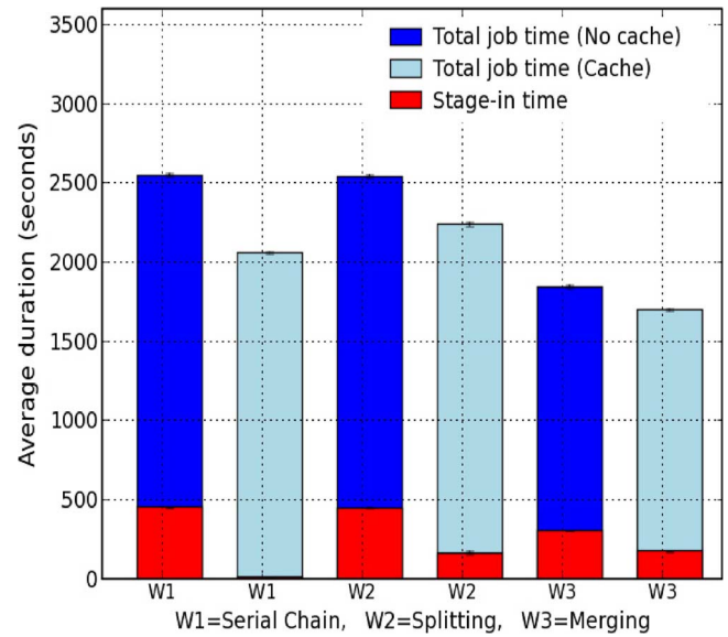
Fig. 10. Average job execution time and stage-in time of each job using data caching and no-caching for different types of workflow executed under high load conditions (d3f3) at SE.
